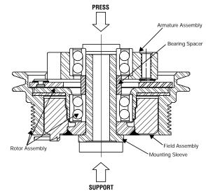
**AWARNING** Support the clutch on the flanged end of the mounting sleeve and only press on the inner race of the bearing to prevent bearing damage. **DO NOT** press on the outer bearing races!
