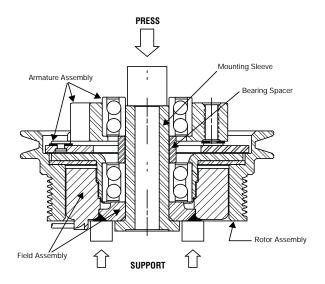
**AWARNING** Support the clutch only in the area shown and only press on the end of the mounting sleeve to prevent bearing damage.
